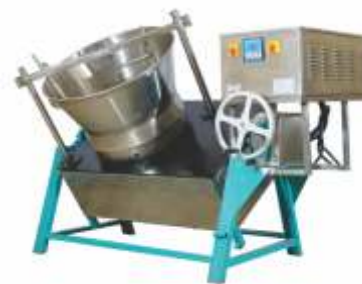
S.S. 304 Induction Khoya/Mawa Machine Tilting / Manual (RANGE 55 LTR. TO 200 LTRS.) POWER : 8KW TO 32 KW
