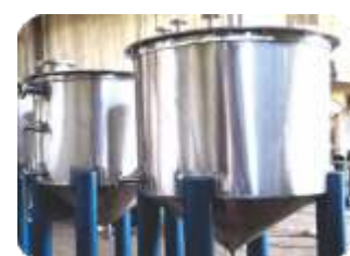
S.S. LIME STORAGE CONE BOTOM-TANK
